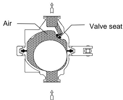
2. When the air has been discharged and water begins to enter the air vent, the float starts to rise due to buoyancy. This pushes it upwards against the valve opening, thus closing the air vent. If there is a rapid rise in water level (caused by rapidly opening a shut-off valve, etc.), a small amount of water may leak with discharged air immediately before the air vent closes.
