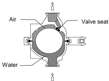
4. When draining the piping, the air vent automatically opens to introduce air and remove water more easily (preventing a vacuum from forming in the piping).
