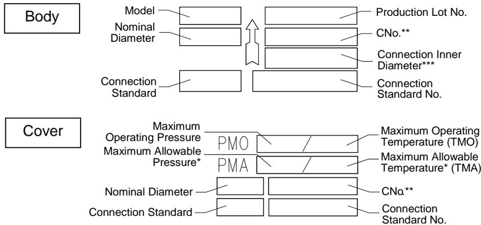
\* Maximum allowable pressure (PMA) and maximum allowable temperature (TMA) are PRESSURE SHELL DESIGN CONDITIONS, **NOT** OPERATING CONDITIONS.
