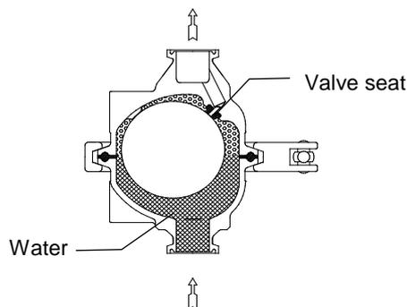
3. When more air is trapped in the air vent due to the inflow of water having closed the valve, the water level in the air vent is forced down and consequently the level of the float falls, opening the valve. Air can now again escape through the air vent, and as it does so the level of the water rises, pushing the float upwards again to close the valve. In this way the VS3 series automatically adjusting air vents constantly respond to the flow of air.
